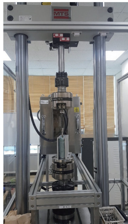
Fig. 2. Pull-out strength test using the MTS system (Bionix 858; MTS systems Corp., Minneapolis, MN, USA). The specimen was mounted on the test jig of a universal material testing machine.
